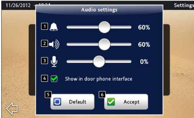
The bell symbol **1** stands for ring tone volume, the speaker symbol **2** stands for the volume of the integrated panel speakers, the microphone symbol **3** stands for setting the built-in microphone's sensitivity.
