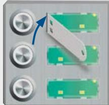
5 Insert the label field on the left side and snap it into place, done.
